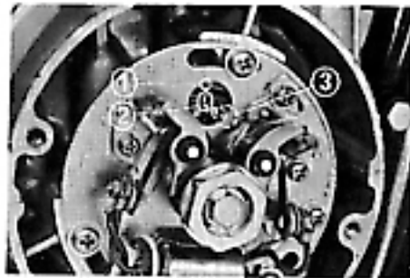
(1) Index mark (2) "T" mark (3) 2.3 cylinder mark
